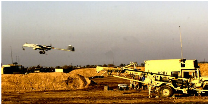
Photo 1: A Shadow TUAV launches from its catapult just prior to an intelligence-gathering mission for 2nd Brigade Combat Team in Baqubah, Iraq. Photo by Sgt. Troy Chatwin. Photo courtesy of ARCENT Public Affairs Office, used with permission.
