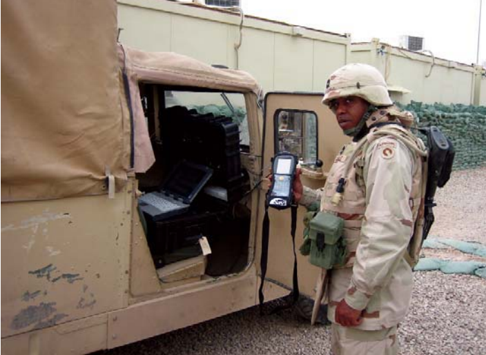
A Soldier in Iraq displays handheld RFID interrogator used to track shipments to the "last tactical mile." (USMC Photo)
